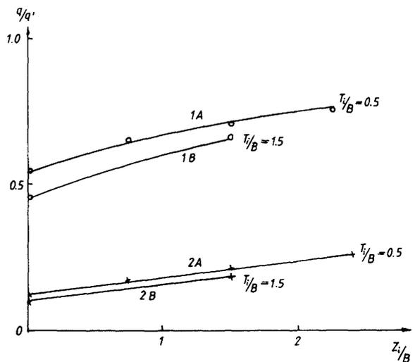
FIG. 8. Relative bearing capacity—depth of weak strata relationship (notation as in Fig. 5).
