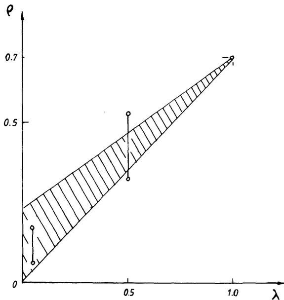
FIG. 7. Bearing capacity ratio ( $\rho$ )—uniaxial strength ratio ( $\lambda$ ) relationship. For definitions see text.
