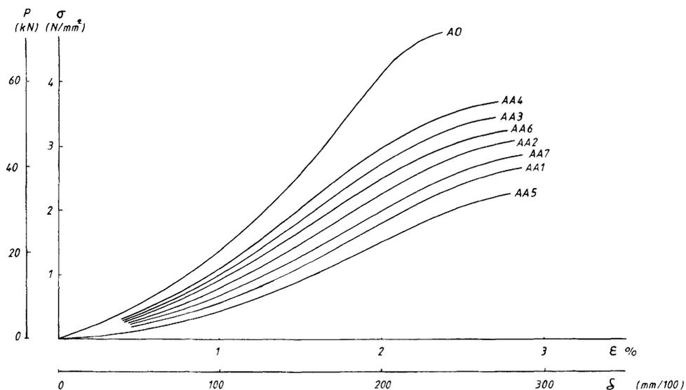
FIG. 3. Load-settlement, stress-strain curves for AA series of tests.
