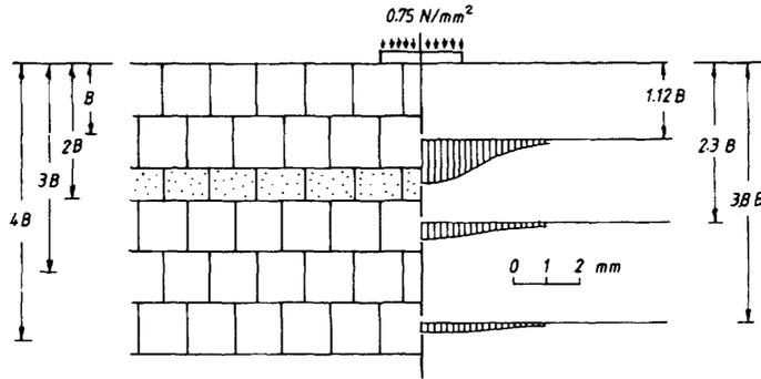
FIG. 6. Typical test deformations (Test AB3).
