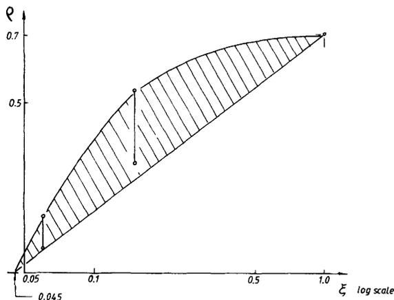
FIG. 9. Bearing capacity ratio ( $\rho$ )–modulus of elasticity ratio ( $\epsilon$ ) relationship.
