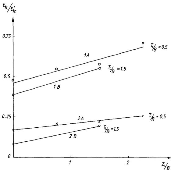
FIG. 5. Relative deformability–depth of weak strata relationship (1A,1B: Material S1 for weak strata; 2A,2B: Material S2 for weak strata). For notation see Fig. 2.
