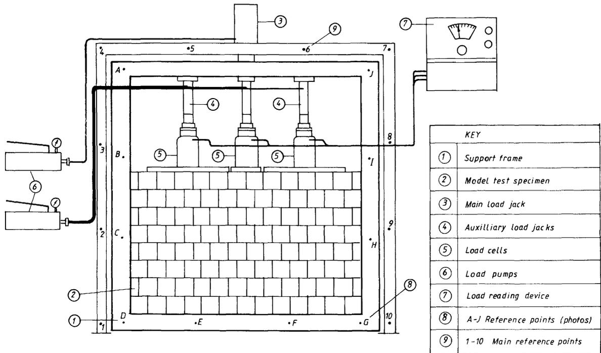
FIG. 1. Loading and monitoring facilities used for the experiments.
