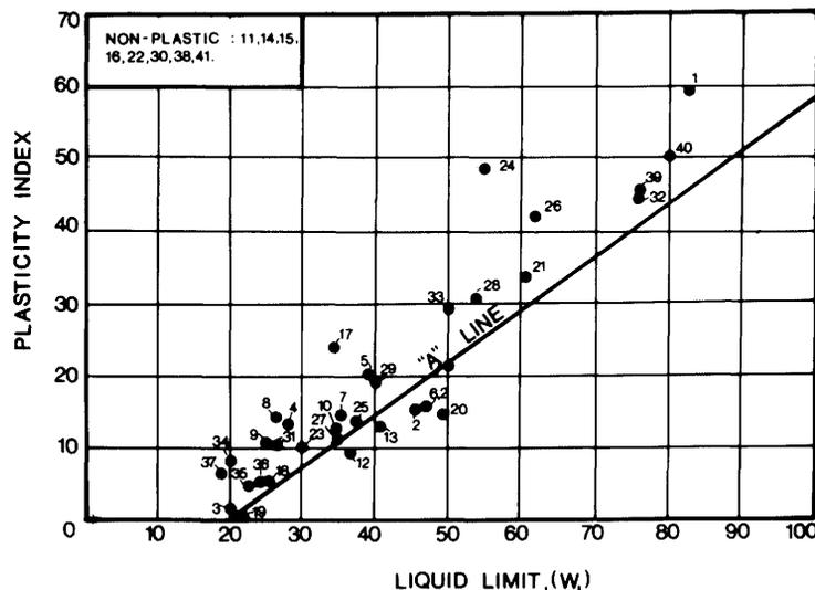
FIG. 3. Casagrande plot of total plastic soil samples with AASHTO (1961) soil groups.
