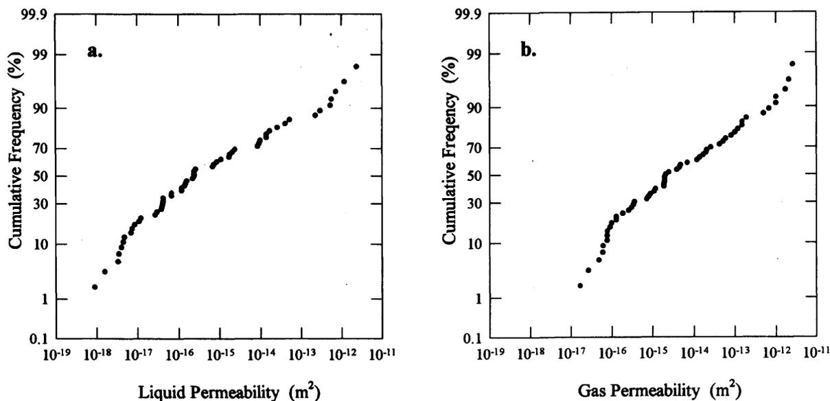
FIG. 1. Cumulative normal probability plots for the log transformed permeability data. (a) cumulative normal probability plot of the liquid permeability data and (b) equivalent plot of the gas permeability data.
